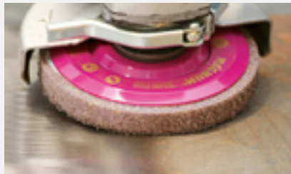
Steel: Fine grinding, deburring, rust removal
