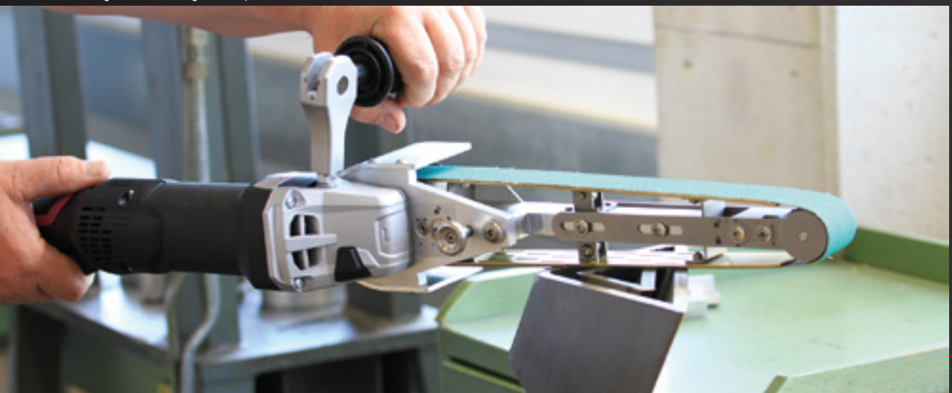
Precise smoothing and deburring of saw parts
