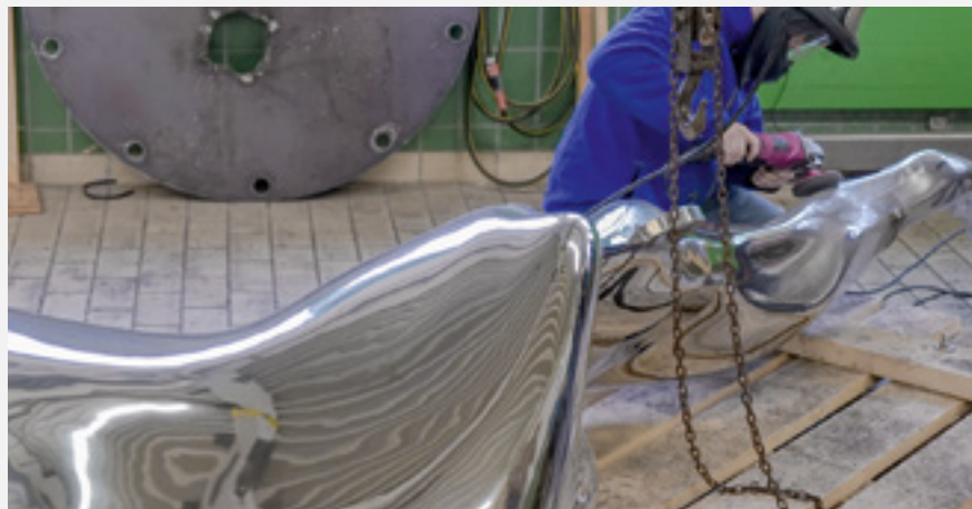
Mirror-finish polishing (here, on stainless steel)
